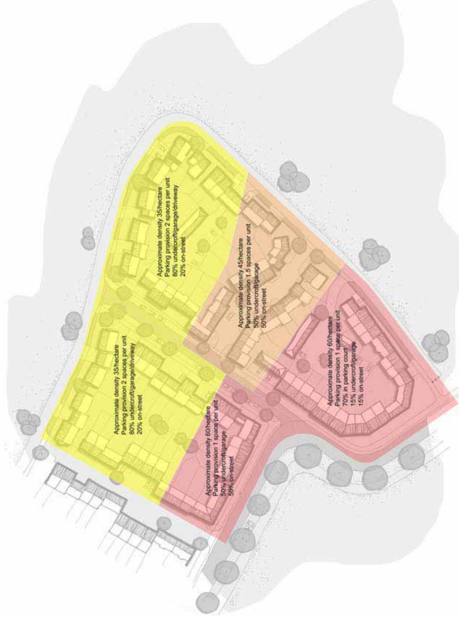
Example block demonstrating how numbers and parking provision can be accommodated within a variety of street typologies and densities.
