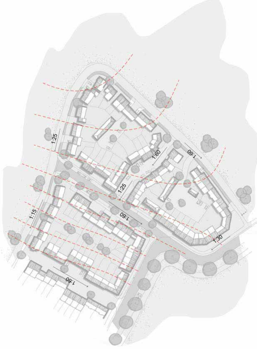
Illustrative plan showing how level changes can be accommodated within a typical development block.
